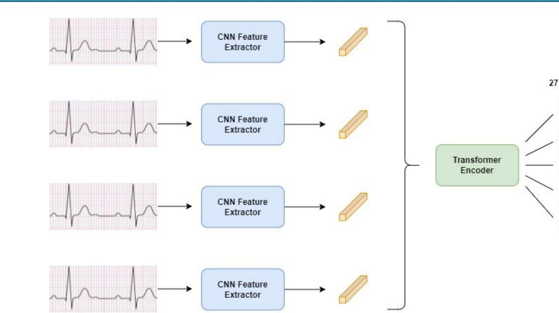
Secondly, we tried dividing each ECG into 5 segments of equal length, which are then passed through CNNs to extract a feature vector. These vectors are then passed through a transformer encoder to achieve our final output classification.
