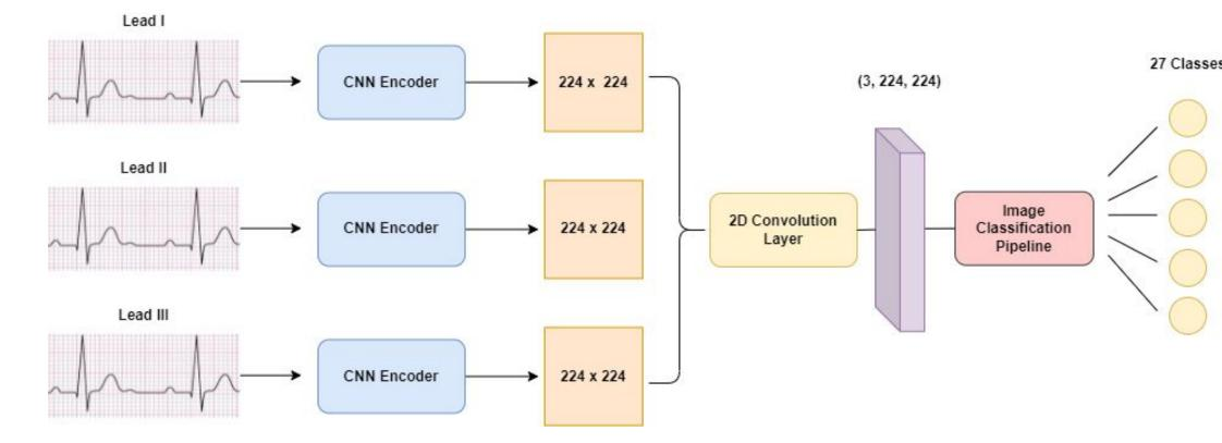
Finally, we applied image classification pipelines on image representations of ECGs. We use CNN encoders to transform each lead into a 2D array, before concatenating them together. We then pass the leads into a 2D convolution to obtain an RGB image representation, and we classify the image into our final output.
