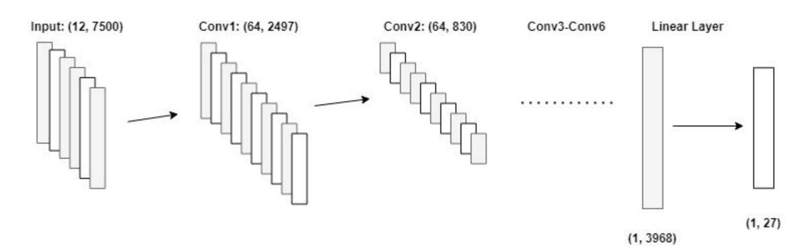
Firstly, we used a standard convolutional neural network (CNN), which runs 1D convolutions across our input ECG to eventually achieve an output layer that classifies the ECG into 1 of 27 diseases.
